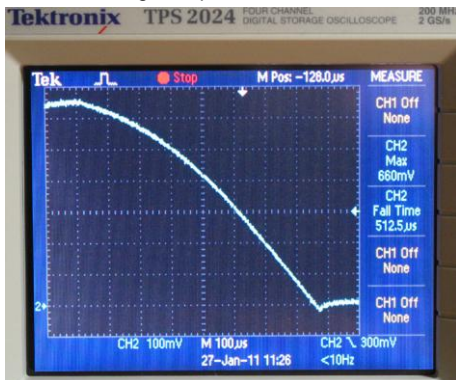
PARAPULSER fall time of magnetic pulse
